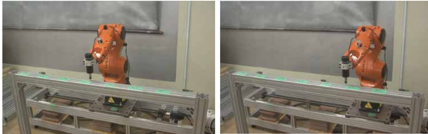
Setting the Robot on the uni-axial traveling rail for expand machining range.
